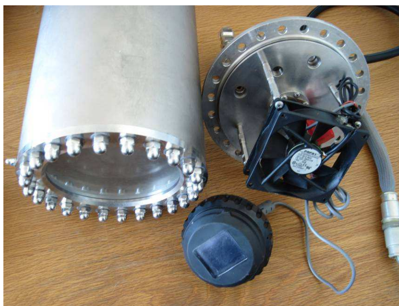
Figure 28: The test fixture used to study the effect of long term 8% CO 2 exposure on cell voltages.
