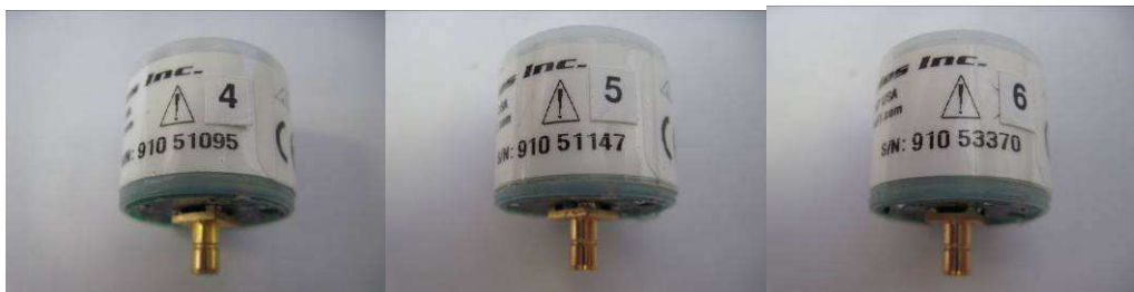
Figure 2 Oxygen sensor test batch N2, manufactured in October 2009, tested in February, March, April 2011 to a Deep Life Procurement Specification [1]. When new, these have an output of nominally 5mV in air. These cells are not temperature compensated internally: they are used with external digital temperature compensation.
