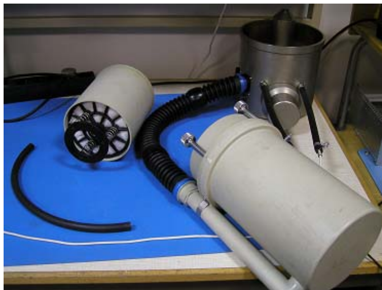
Fig 4-8. CBM with empty scrubber canister and curved tube.
