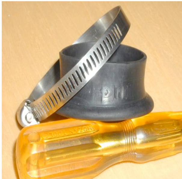
Fig 1:: Hose with jubilee clip, after tensioning the clip until the grub screw failed, then tensioning the hose until the hose failed. Hose failure point is at the same point observed in the tests reported in the FMECA Vol 4
